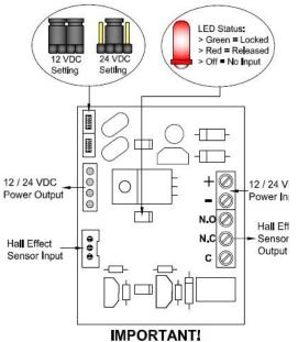
Set the jumper position according to the power input correctly before switch ON the power.
