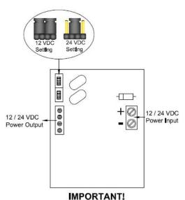
Set the jumper position according to the power input correctly before switch ON the power.
