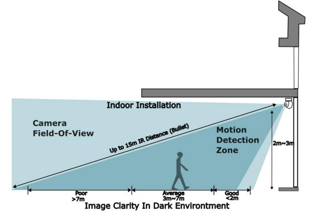
\*\* Dark Knight IP Camera IR distance can up to 20meter. For the motion detection zone distance can up to 12m. For the average clarity of the image during night time recording can up to 7m. A good recommendation installation height up to 3m height
