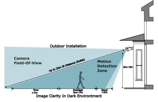
\*\* Dark Knight IP Camera IR distance can up to 20meter. For the motion detection zone distance can up to 12m. For the average clarity of the image during night time recording can up to 7m. A good recommendation installation height up to 3m height
